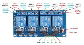
Fig-7: 4 - Channel Relay Module
