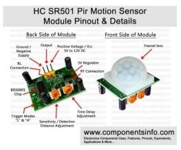
Fig-4: Passive Infrared Sensor
