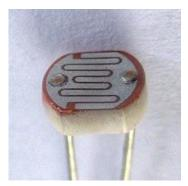
Fig – 3: Light Dependent Resistor Sensor
