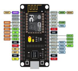
Fig – 5: Node MCU Controller (ESP8266)
