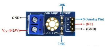
Fig-1: Voltage Sensor
